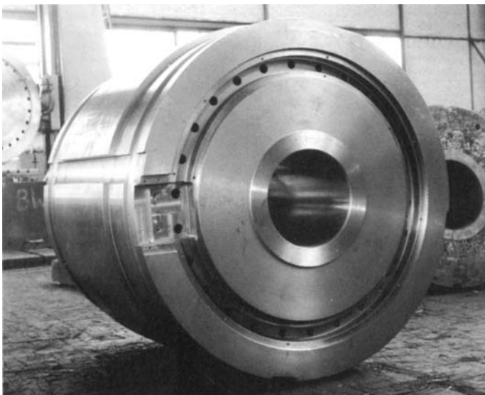
Fig. 10 Round container with liner. Source: Edelstahlwerke Buderus AG
