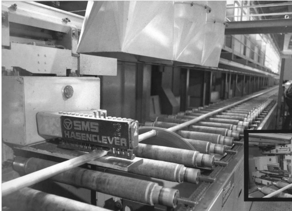
Fig. 29 Double-puller system and flying hot saw. (1) Double-puller system. Source: SMS Engineering Inc.
