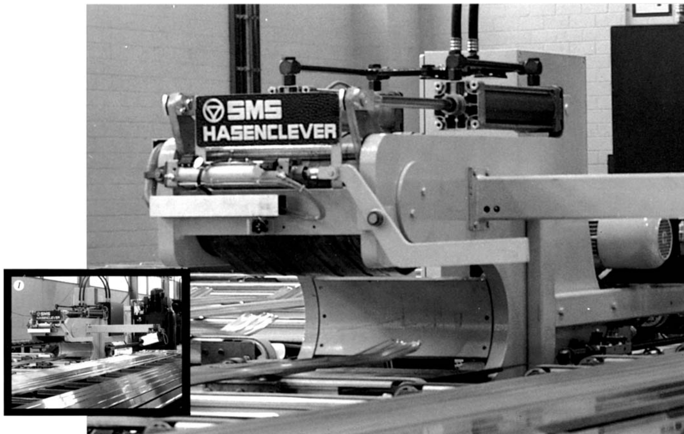
Fig. 30 Stretcher tailstock. (1) Stretcher headstock. Source: SMS Engineering Inc.
