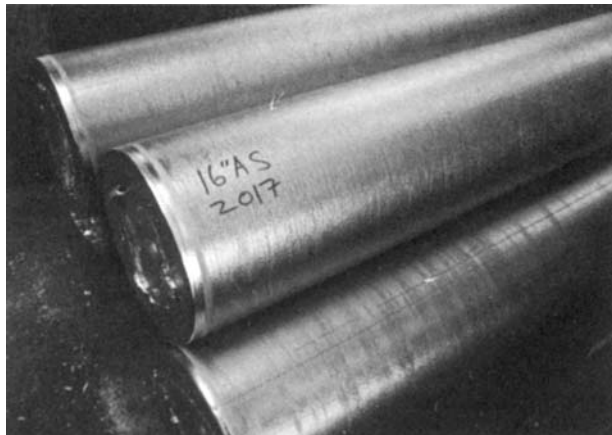
Fig. 14 AirSlip as-cast 2017 billet surface. Source: Ref 3
