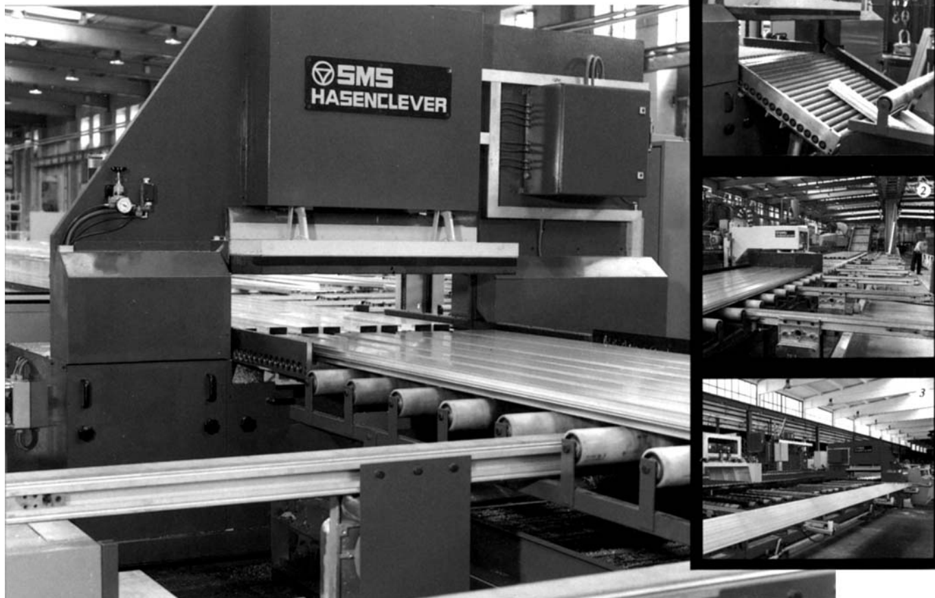
Fig. 31 Saw with hold-down device and discharging belts. (1) Saw, table with driven rollers, and transport for section ends. (2) Adjustable saw contact for exact positioning of the bundled sections. (3) Saw with section contact and discharging belts. Source: SMS Engineering Inc.
